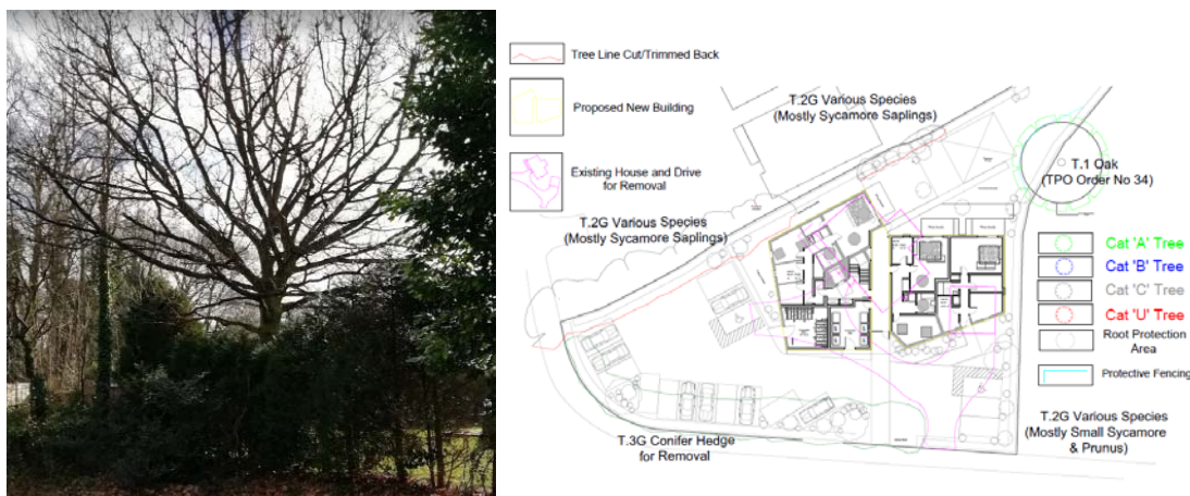
Fig K – Picture of TPO Oak tree and plan showing trees location relative to development.
